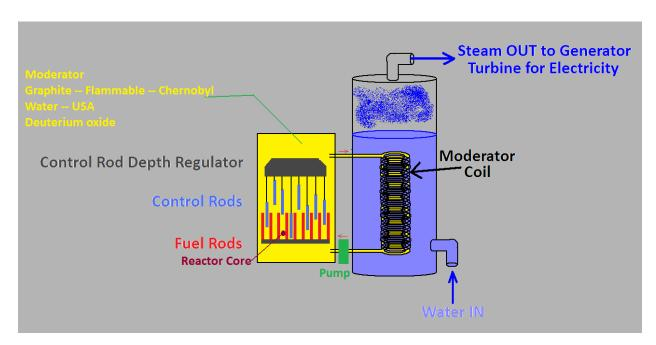
Control Rods are made from neutron absorbing metals: Cd and B. Too few neutrons in the raector core and reaction dies out. Too many neutrons and get core overheating: the core melts down and maybe thermonuclear explosion (SAFETY SYSTEMS!)
