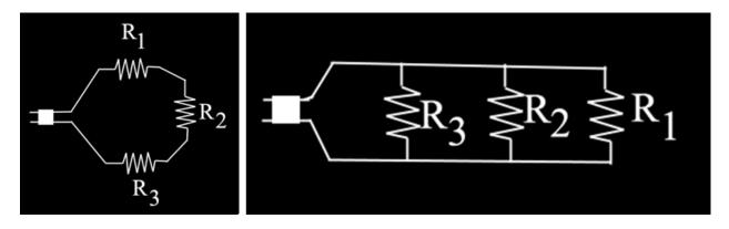
Series (left) – set up like X-mas lights: one goes out, they all go out – Greatest  $\Omega$  (resistance to electron flow), least electron flow.
