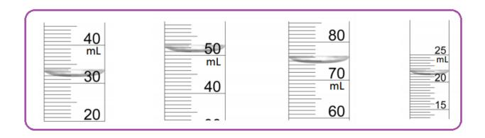
50) Using the diagram above, determine the correct volume to the correct number of sig figs – using the bottom of the meniscus – for each measurement, above. What is a meniscus? Use your own words to define what a meniscus is.
